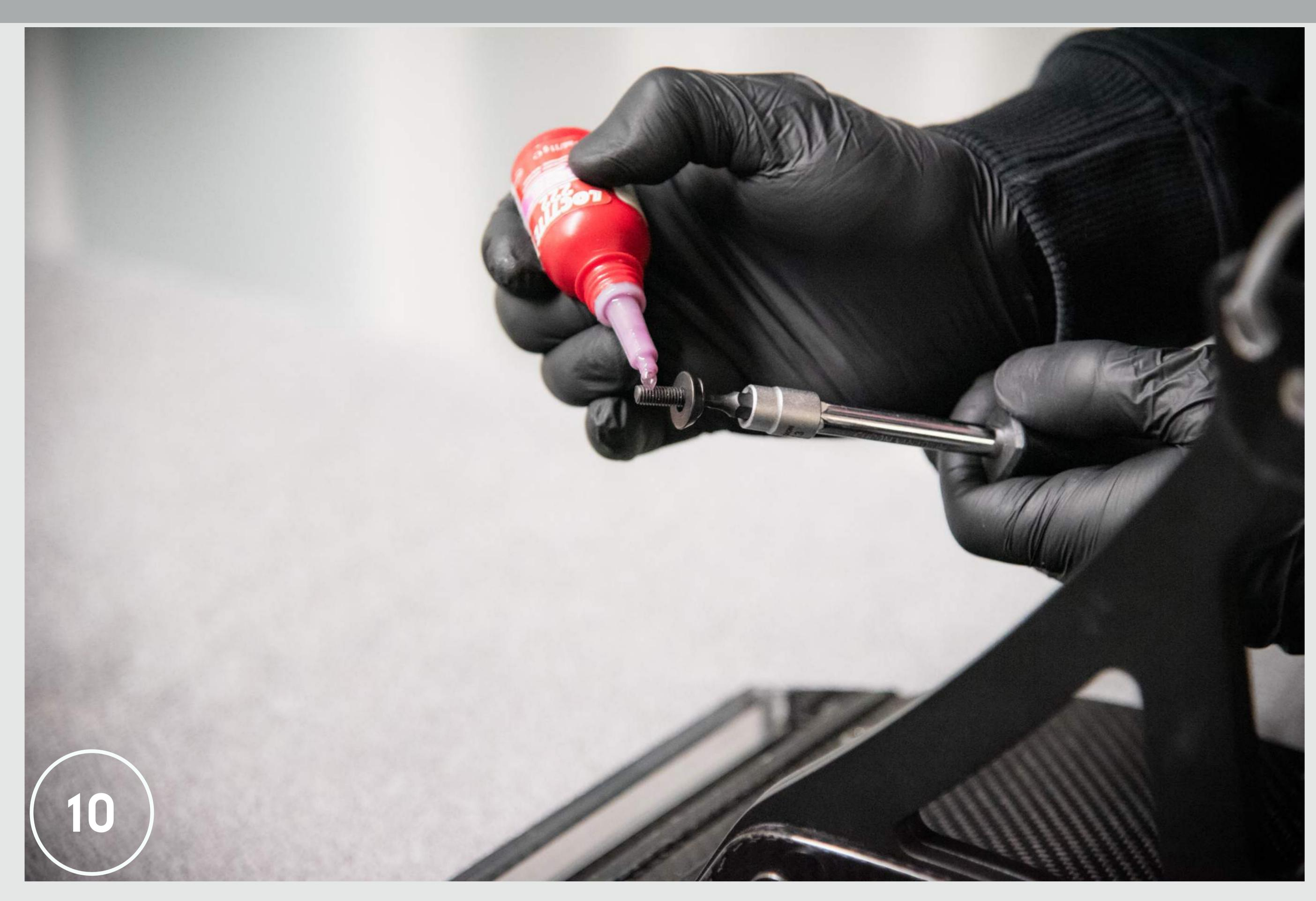
10. Attach the mounting brackets to the spoiler. Apply a low-tear locking adhesive to the mounting screws thread.
