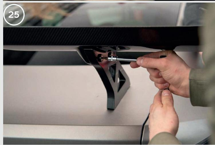
25. If it is even, tighten the screws securing the spoiler to the brackets firmly.
