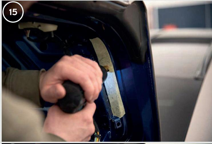
14. Drill the sheet metal layer according to the marked points inside the tailgate.
