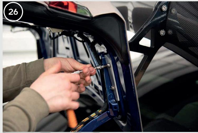
26. Tighten the screws securing the brackets to the tailgate.
