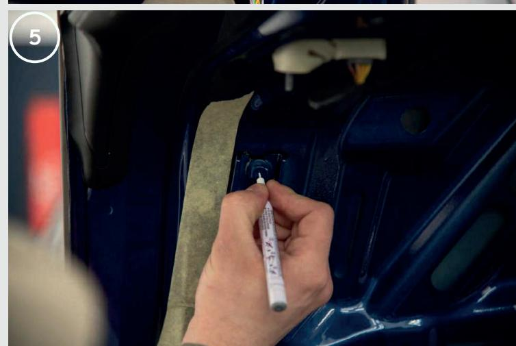
4. Mark the center of the tailgate mounting bolt.
