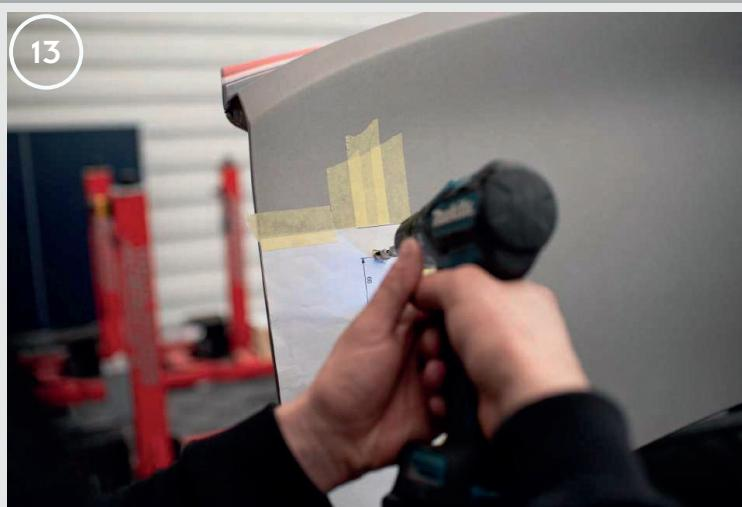
12. Place the form on the tailgate and attach it carefully.
