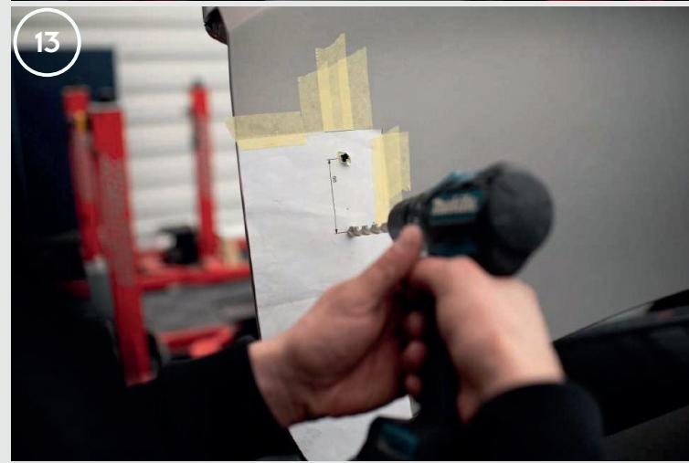
13. Drill holes according to the marks on the form.
